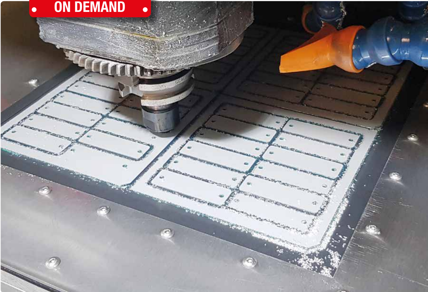
Production facility for customer-specific "Label on demand" label plates
